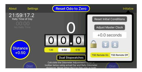
To reset conditions, simply touch the "Reset Initial Conditions" button. The padlock will close and you may see some numbers or objects on the startup screen change.
